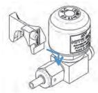
Mount the valve Lock Assist component.
